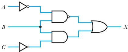
**23.18** Design a logic circuit to take three inputs – *A*, *B* and *C* – and produce a single output *X*, such that *X* is true if, and only if, precisely two of its inputs are true.
