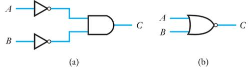
**23.8** Simulate the pairs of circuits in Exercises 23.6 and 23.7 and confirm that each pair produces the same output for every possible combination of the inputs.
