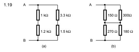
(a) This is  $(1k\Omega + 1.2 k\Omega)//(3.3 k\Omega + 1.5 k\Omega) = 2.2 k\Omega//4.8 k\Omega = 1.51 k\Omega$ .
