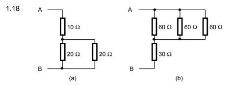
(a) This is 10  $\Omega$ , in series with 20  $\Omega$ //20  $\Omega$ , which is 10  $\Omega$  + 10  $\Omega$  = 20  $\Omega$ .
