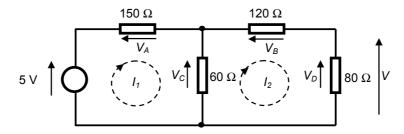
The circuit contains two meshes. To these, we assign loop currents  $I_1$  and  $I_2$  as shown above. The diagram also defines the various voltages.
