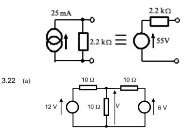
With just the 12 V source (and the 6 V source replaced by a short circuit)  $V = 12 \times ((10//10)/((10//10) + 10)) = 4$  V.
