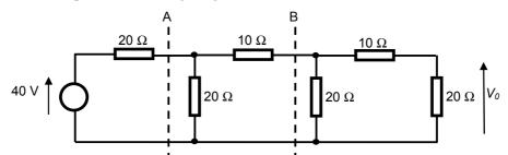
The circuit to the left of the dotted line 'B' can then be replaced by its Thévenin equivalent circuit giving:
