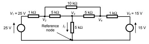
First, we pick our reference node, and label the various node voltages, as shown above. Next we sum the currents flowing into the nodes for which the node voltages are unknown. This gives
