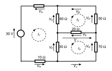
The circuit contains three meshes. To these, we assign loop currents  $I_1$ ,  $I_2$  and  $I_3$ , as shown above. The diagram also defines the various voltages.
