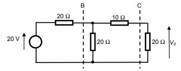
The circuit to the left of the dotted line 'C' can then be replaced by its Thévenin equivalent circuit giving:
