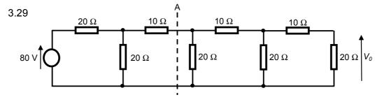
This circuit can be analysed in many ways. One attractive method is to use Thévenin's theorem to replace parts of the circuit with simpler arrangements.
