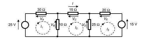
The circuit contains three meshes. To these, we assign loop currents  $I_1$ ,  $I_2$  and  $I_3$ , as shown above. The diagram also defines the various voltages.
