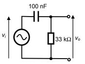
T =  $CR = 100 \times 10^{-9} \times 33 \times 10^{3} = 3.3$  ms.  $\omega_{c} = 1/T = 1/3.3$  ms = 303 rad/s.  $f_{c} = \omega_{c}/2\pi = 303/2\pi = 48.2$  Hz. This is a low-frequency cut-off.
