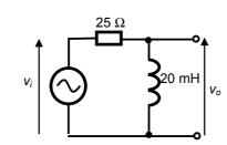
T = L/R = 20 × 10<sup>-3</sup>/25 = 800 µs.  $\omega_c$  = 1/T = 1/(800 × 10<sup>-6</sup>) = 1,250 rad/s.  $f_c$  =  $\omega/2\pi = (20 \times 10^3)/2\pi = 199$  Hz. This is a low-frequency cut-off.
