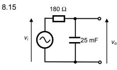
T =  $CR = 25 \times 10^{-3} \times 180 = 4.5$  s.  $\omega_c = 1/T = 1/4.5 = 0.222$  rad/s.  $f_c = \omega_c/2\pi = 0.222/2\pi = 35.4$  mHz. This is a high-frequency cut-off.
