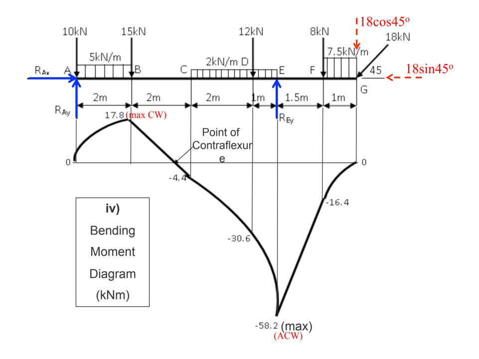
v) The point of contraflexure (or inflexion) occurs at the point along the beam span where M = 0.  $18\cos 45^{\circ}$ 10kN 8kN 15kN 12kN 18kN 7.5kN/m Х 5kN/m 2kN/m D 18sin45° B ٦E F RAY G 1.5m 2m 2m 2m 1m .m  $\mathsf{R}_{\mathsf{Ay}}$ 17.8 Rev 23.9kN Point of Contraflexur е 0 Ο x (m) -16.4 Defining the distance from RHS to the point where M = 0 as 'x': -30.6  $M_x = 0 = 23.9x - 10x - (5x2)(x-1) - 15(x-2)$ = 23.9x - 10x - 10x + 10 - 15x + 30= -11.1x + 40i.e., x = 3.6 m
