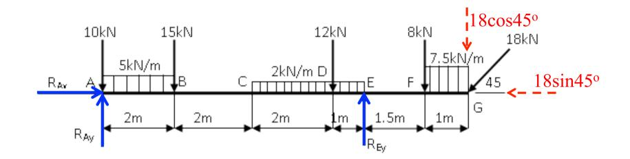
Applying 2D force equilibrium in X-direction:  $\sum F_x = o$   $R_{Ax} - (18\sin 45^\circ) = 0 \quad \boxtimes \quad R_{Ax} = 12.7 \text{ kN}$
