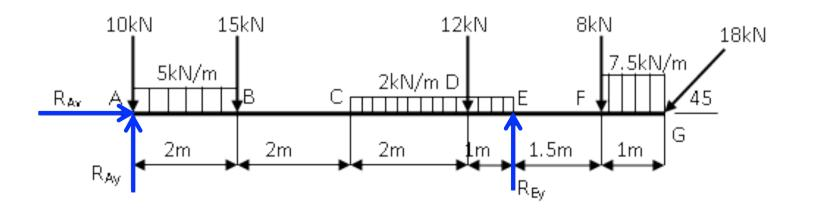
**i)** The pin support at A provides 2 force reactions (horizontal and vertical), and the knife edge at E provides a vertical reaction only.
