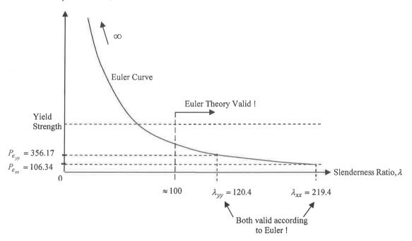
**Note:** It is always useful to produce an axial compressive load v. slenderness ratio graph showing the Euler curve, the yield line and the validity limit of Euler. In addition, the inclusion of the actual  $\lambda$  values obtained from a design problem along with the corresponding P values helps to illustrate Euler Theory and its proper application.
