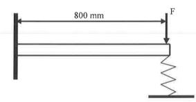
Note: The max. deflection at the free end of a cantilever is found from:
