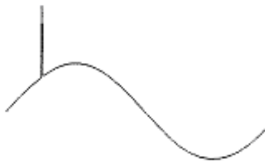
Figure 2 The waveform of a typical lightning impulse
