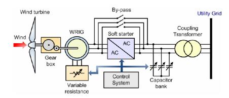
Gearbox: Used for speed transmission from slow rotor hub speed to high generator speed.
