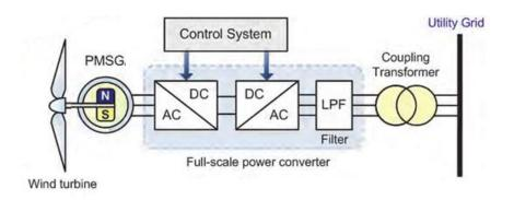
**PMSG**: Used to convert mechanical power to electrical power without the use of gearbox. Typically the rotor hosts large number of permanent magnet poles to allow operation at low speed. The stator windings directly connected to the constant-frequency three-phase grid, rotor circuit connected to back-to-back power converters
