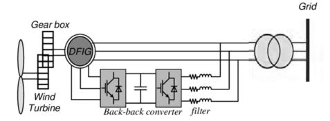
Gearbox: Used for speed transmission from slow rotor hub speed to high generator speed.
