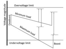
2) A renewable DG is connected to an 11-kV feeder. The resistance between the DG source and the feeder bus is 5 ohms and the overvoltage limit is 105%. Assuming the bus voltage is nominal and constant before the DG is installed, estimate the maximum power rating of the DG in terms of overvoltage limit. (when there is no reactive power generation or consumption)
