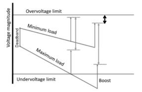
DG can give rise to voltage rise. There has to be sufficient overvoltage margin to ensure such voltage rise will not lead to an overvoltage.
