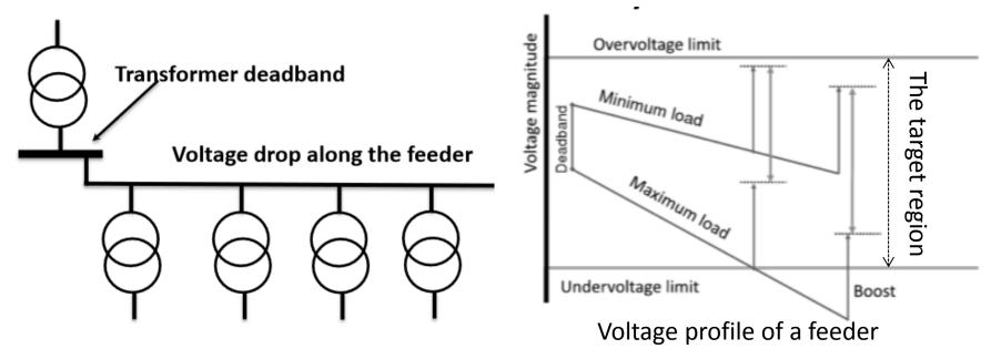
Image by Chapter 5, Bollen, Math H. J., < Integration of distributed generation in the power system >, 2011
