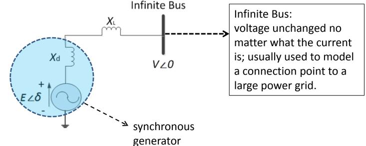
A Synchronous Generator (SG) based DG is connected to an infinite bus through a transformer and a transmission line with a total reactance of XL.
