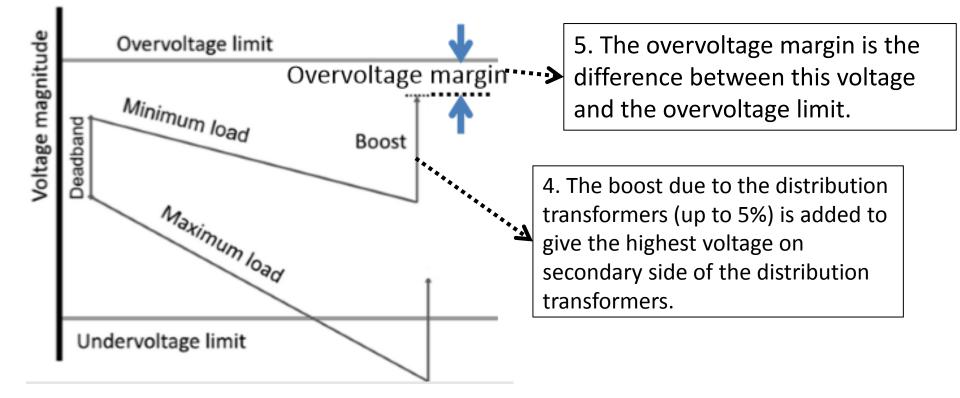
Image by Bollen, Math H. J., <Integration of distributed generation in the power system, Chapter 5> 6. The HC is proportional to the margin in terms of overvoltage.
