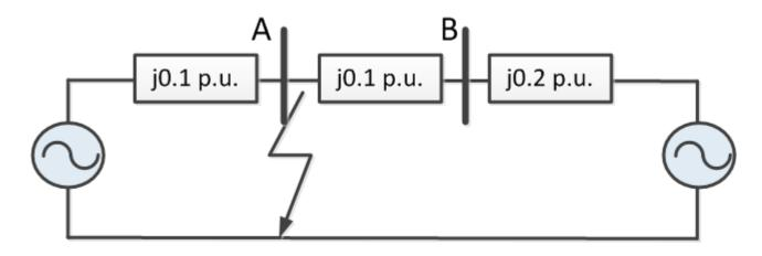
The equivalent circuit for fault calculation is shown above. The large power system has been replaced by its Thevinin equivalent with the impedance. Since the network operates at nominal voltage and the load current is assumed negligible, both voltage source has been set at 1.0 p.u.. The magnitude of the fault current at Bus A is given by
