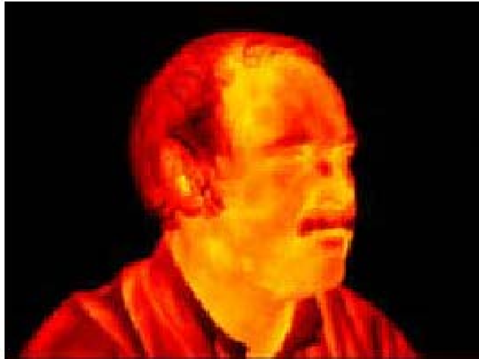
IR Image acquired with a 320 x 240 element QWIP matrix
